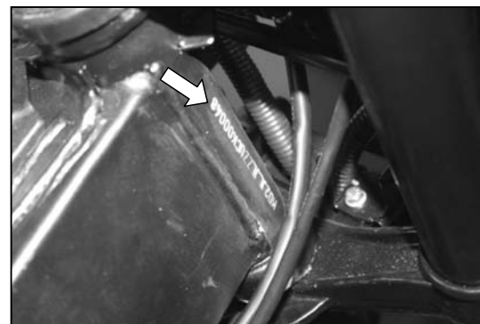
Engine Number Location On LH Side Crankcase Near Gear Change Lever (Alpha-Numeric - 11 Digits)
