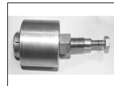
Front fork oil seal & antifriction bush extractor tool
